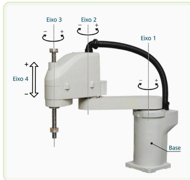
Figura 4.5: Robô SCARA
